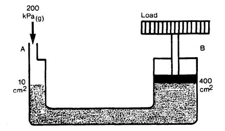
The pressure on the surface of the fluid is the same in the left cylinder as in the right hand cylinder.
