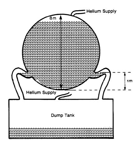
The pressure in the goose neck is the pressure of helium in the dump tank. The pressure at this point is also equal to the pressure due to the weight of heavy water plus the cover gas pressure.
