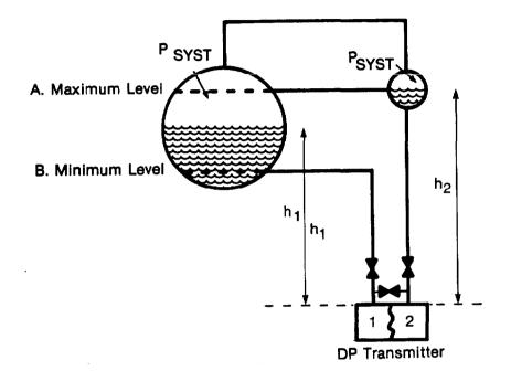
To provide a test reading corresponding to the maximum level in the tank we must provide a zero differential pressure at the transmitter.
