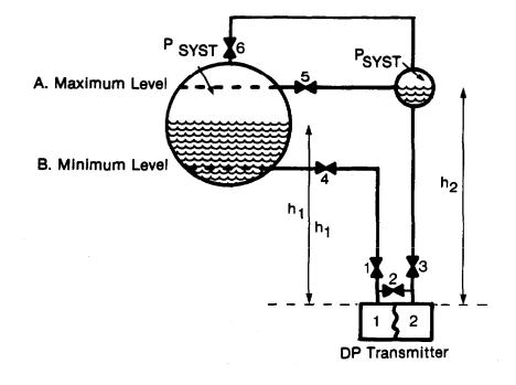
Before considering valve positions etc, an important point to note is that the DP cell is only designed to measure a differential pressure representative of the liquid height in the drum, (ie, a few metres, say 100 kPa). No operation should allow one side of the cell to be depressurized while the other side remains under full system pressure, (ie, liquid pressure and steam pressure  $\simeq 4$  MPa) which would over pressurize the pressure sensing element.
