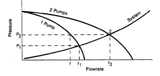
Under the original conditions we have two pumps producing a system flowrate of  $f_2$  which is <u>equally</u> shared by the pumps with a discharge pressure of  $P_2$ . The operating point is 2 on the head curves.
